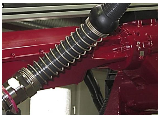
Passives Federrückholssystem Passive spring retract system
